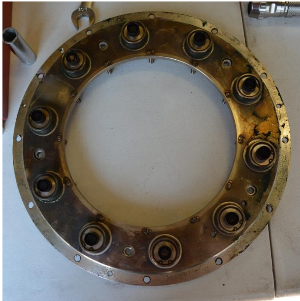
Inside of fuel manifold/reader combustor case showing 10 spill-type burners
