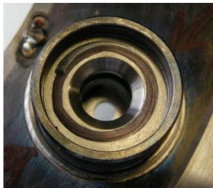
Inside of fuel manifold/reader combustor case showing 10 spill-type burners
